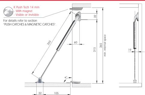
The dimensions of the drilling plan refer to carcases which use standard unsprung hinges and mounting plates 0 mm. Please note that the  $\alpha^{\circ}$  opening angle shown data is purely indicative. It varies with respect to the hinge brand and adjustment carried out.
