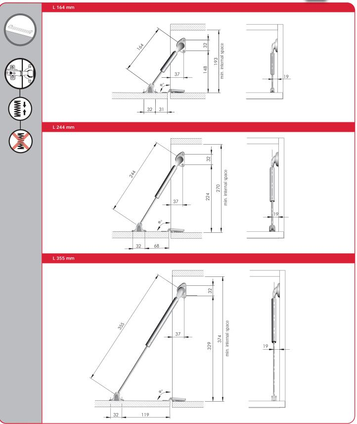
The dimensions of the drilling plans refer to carcases which use *standard sprung hinges* and mounting plates 0 mm. Please note that the  $\alpha^{\circ}$  opening angle shown data is purely indicative. It varies with respect to the hinge brand and adjustment carried out.
