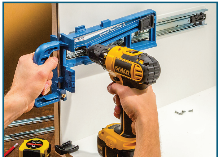
Fig. 2 - The handle provides a comfortable, secure grip for holding the slide in perfect alignment while you drive the mounting screws
