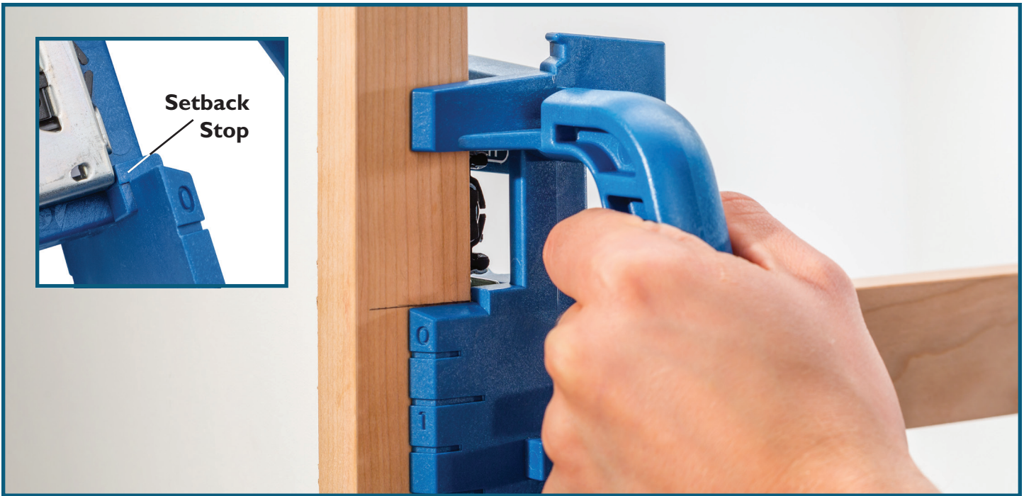
Fig. 1 - Easy alignment: Match the bevel to your mark. The jig includes notches that allow you to offset the slide mounting location
