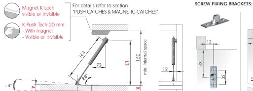
Opening angle adjustment is possible only with K12 SYSTEM ADJ version.
